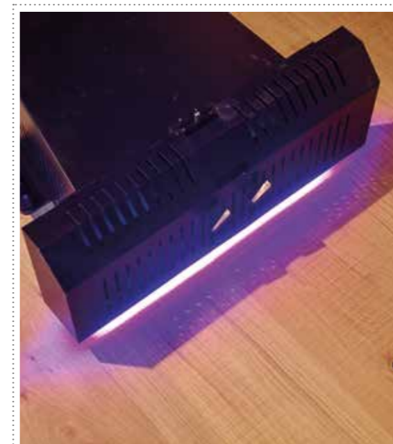
LED-curing on-site unit
